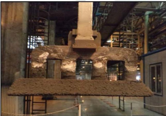
Figure 3: Clean anode butt in good condition.
