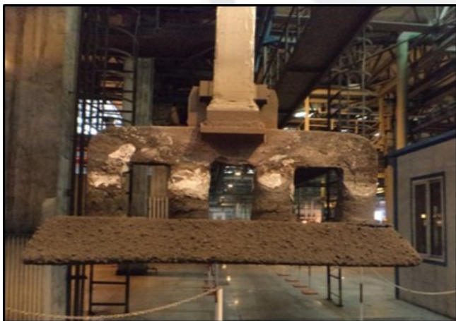
Figure 3: Clean anode butt in good condition.
